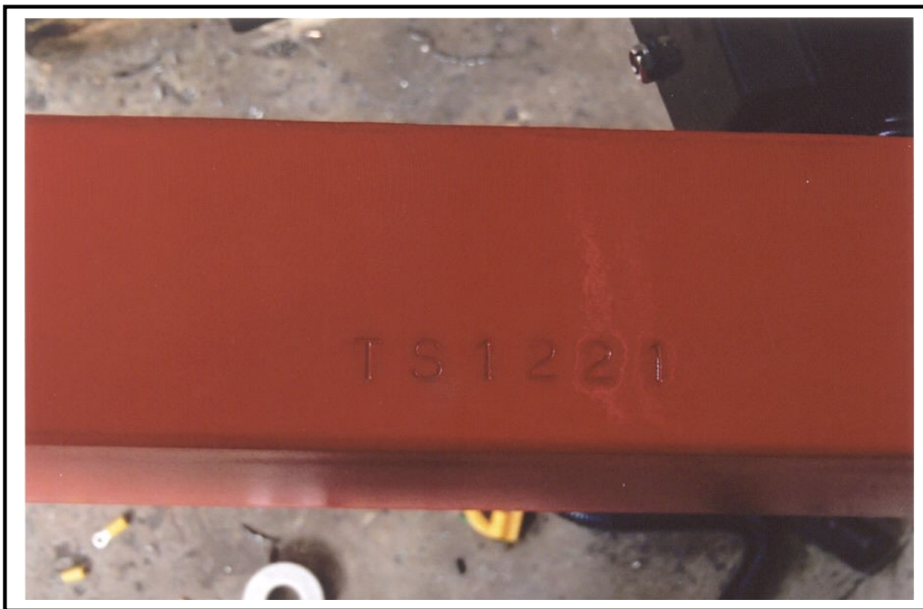
Identification (VIN) Number stamped on frame of trailer
